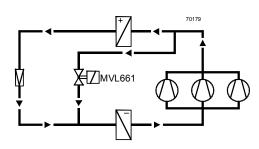
Suitable for use in large refrigeration systems in air conditioning plant, to prevent unacceptable temperature fluctuations between the compressor stages.
