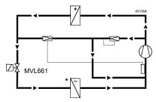
b) Refrigerant valve MVL661..-.. for capacity control of a chiller.
