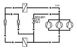
Suitable for large refrigeration systems in air conditioning applications with several compressors or compressor stages, and where the evaporator and compressor are some distance apart (attention must be paid to the oil return).
